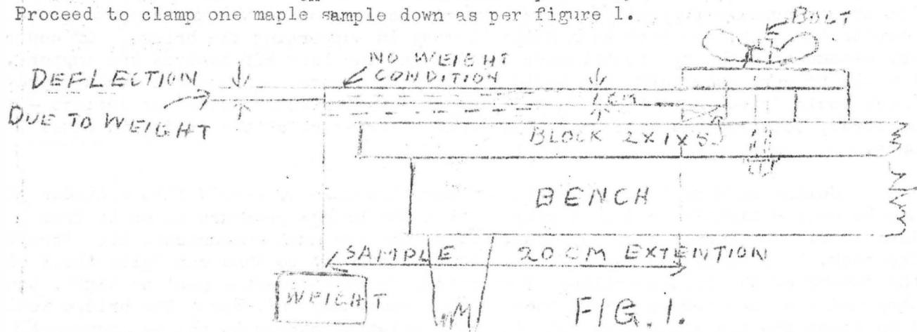
The sample must be perfectly horizontal. After the weight has been hung as shown, measure the sag or deflection of the sample very carefully. Remove maple sample.
