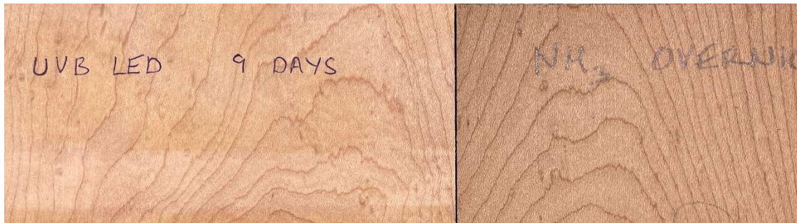
Figure 5: Maple exposed to LED UVB for 9 days (L) and overnight in an ammonia atmosphere (R).
