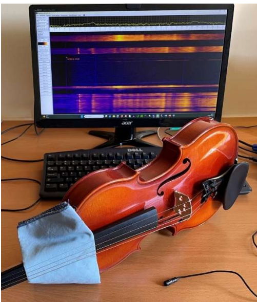
Figure 3: Measuring the signature mode frequencies of a 1992 Karl Höfner.
